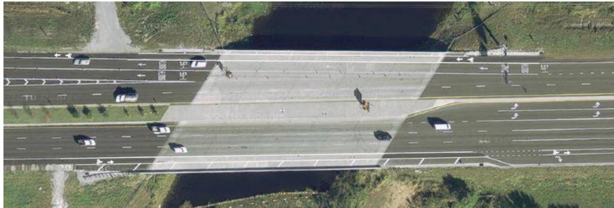
Figure 5A.14: Proposed treatment to facilitate bicyclists crossing of bridge
