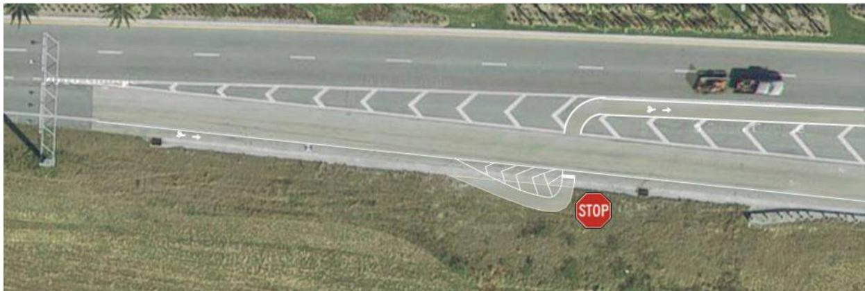
Figure 5A.12: Proposed treatment to facilitate bicyclists crossing of on-ramp
