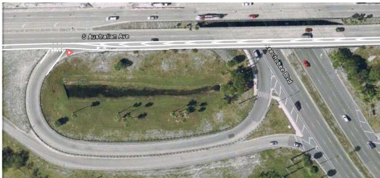
Figure 5A.7: A gap acceptance slip lane could allow for a bike lane across the overpass
