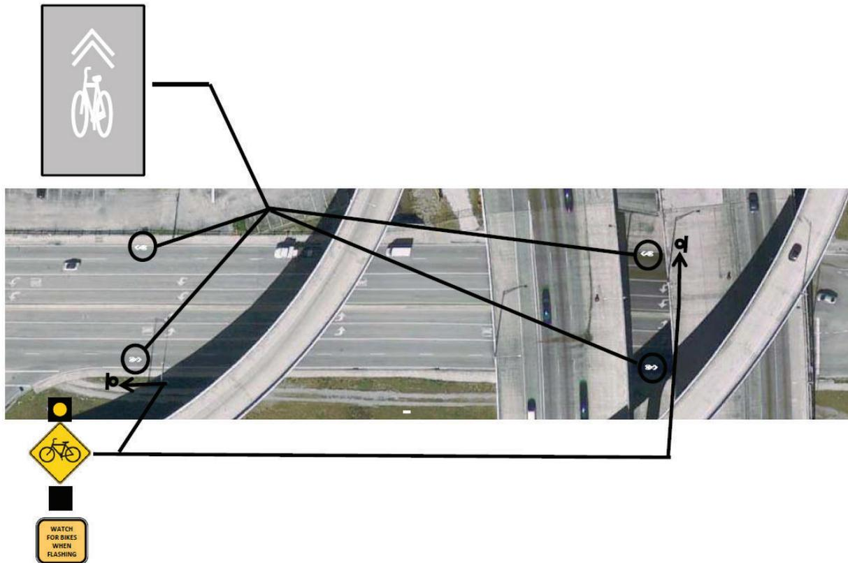
Figure 5A.18: Proposed Shared Lane Markings and activated warning signs under I-95 overpass
