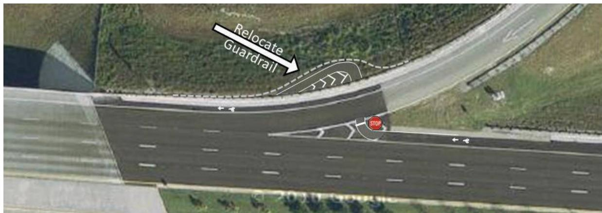
Figure 5A.15: Proposed treatment to facilitate bicyclists crossing of off-ramp
