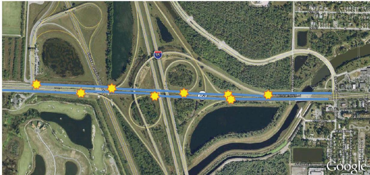
Figure 5A.11: There are eight conflict points between turning or exiting motor vehicles and bicyclists using the shoulders.
