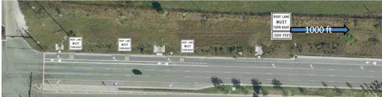
Figure 5A.16: Proposed treatment to facilitate through moving bicyclists at intersection with Turnpike Plaza
