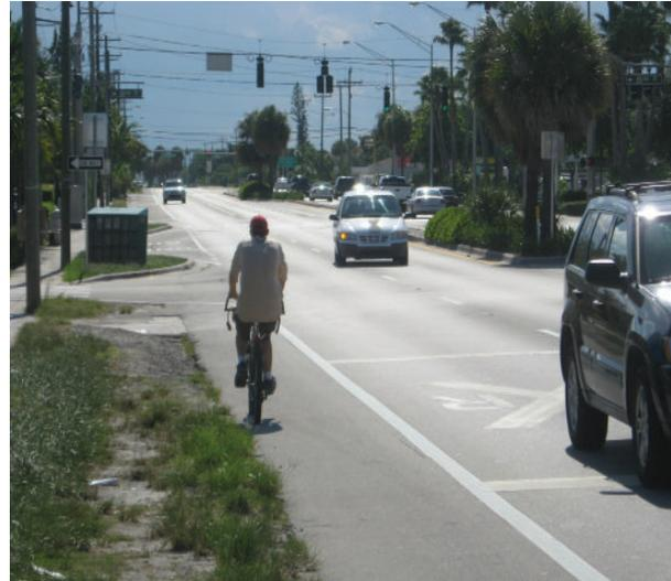
Figure 5A.20: Curbs at bus pull-outs encroach on the bike lane just between Akron and Erie Streets
