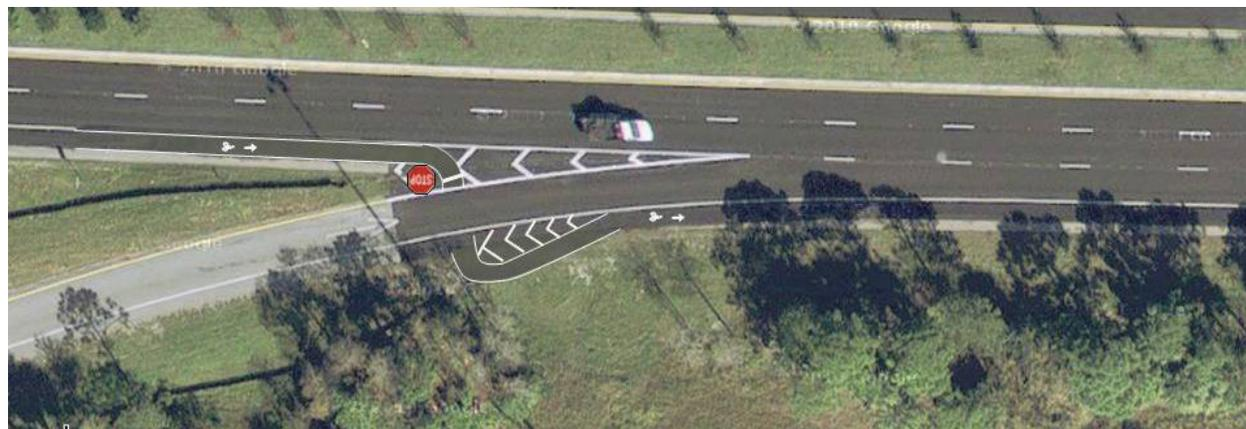
Figure 5A.13: Proposed treatment to facilitate bicyclists crossing of off-ramp
